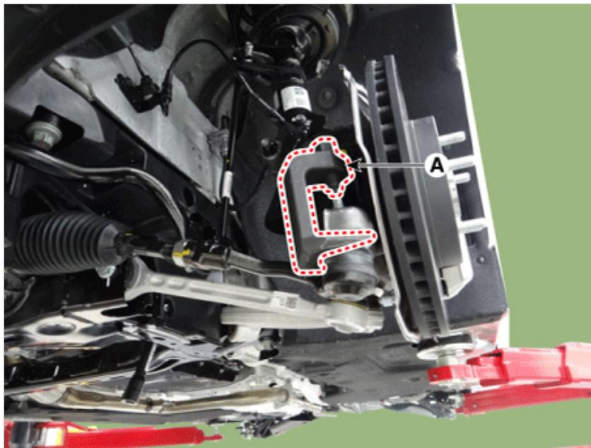
14. Loosen the screw, and then remove the brake disc.
