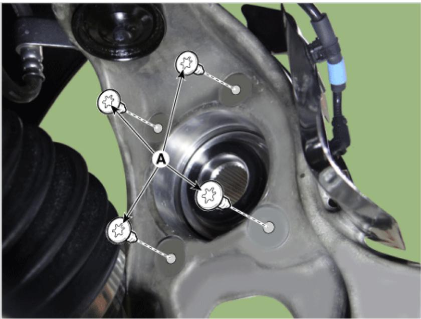
14. Loosen the wheel speed sensor bolt (A) and then disconnect the wheel speed sensor.
