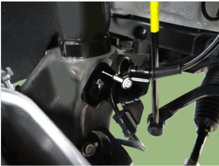
18. Loosen the brake caliper hose bracket bolt.
