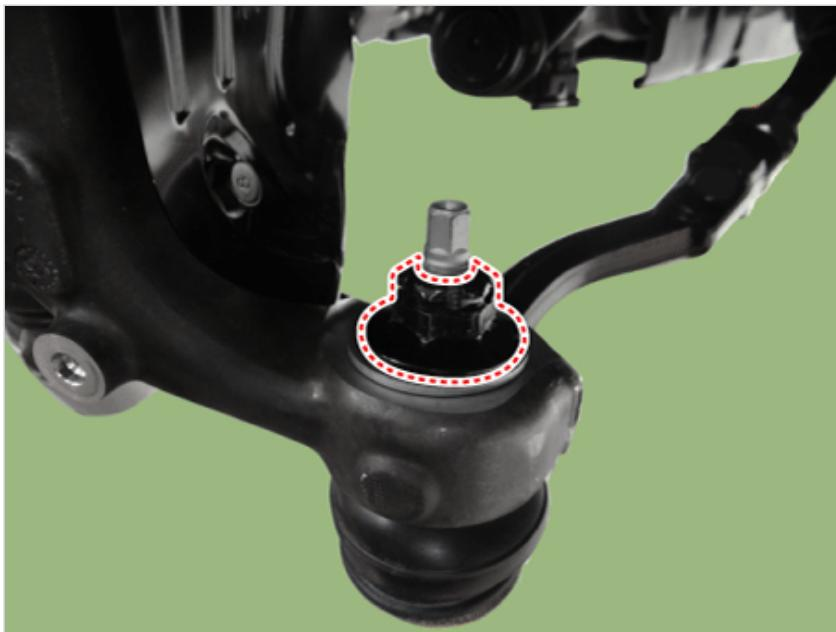
8. Remove the knuckle by using the ball joint remover (A).
