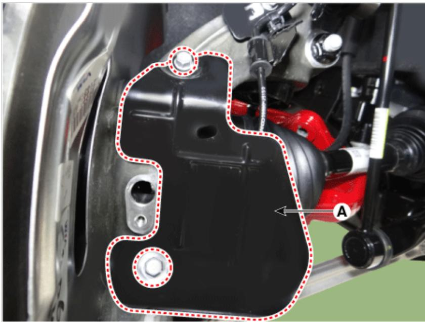
16. Remove the wheel speed sensor bracket (A).
