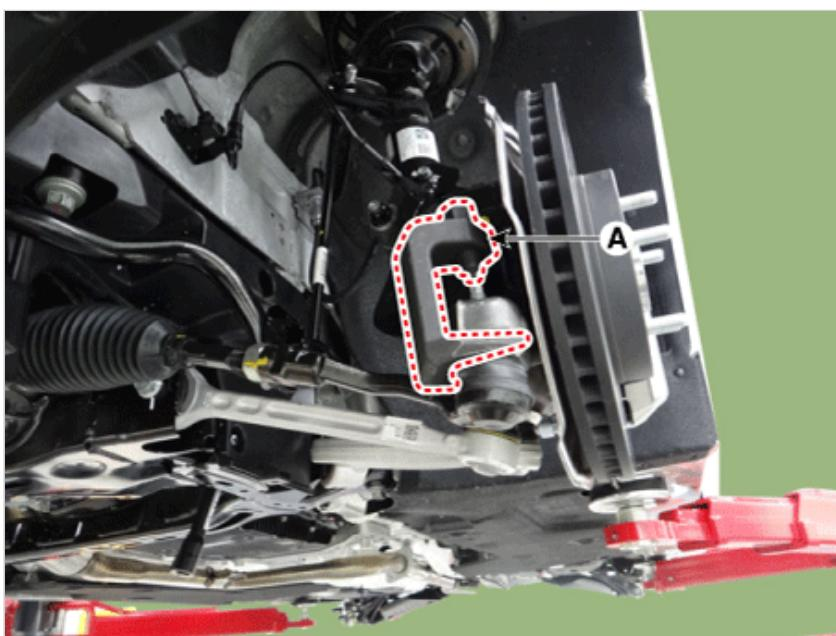
9. Remove the brake hose bracket (A).
