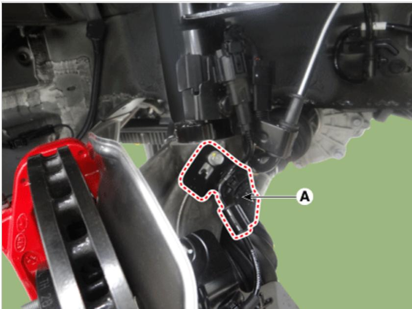
17. Loosen the knuckle upper bolt & nut.
