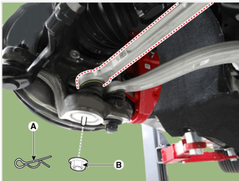
4. Remove the lateral arm by using the ball joint remover (A).
