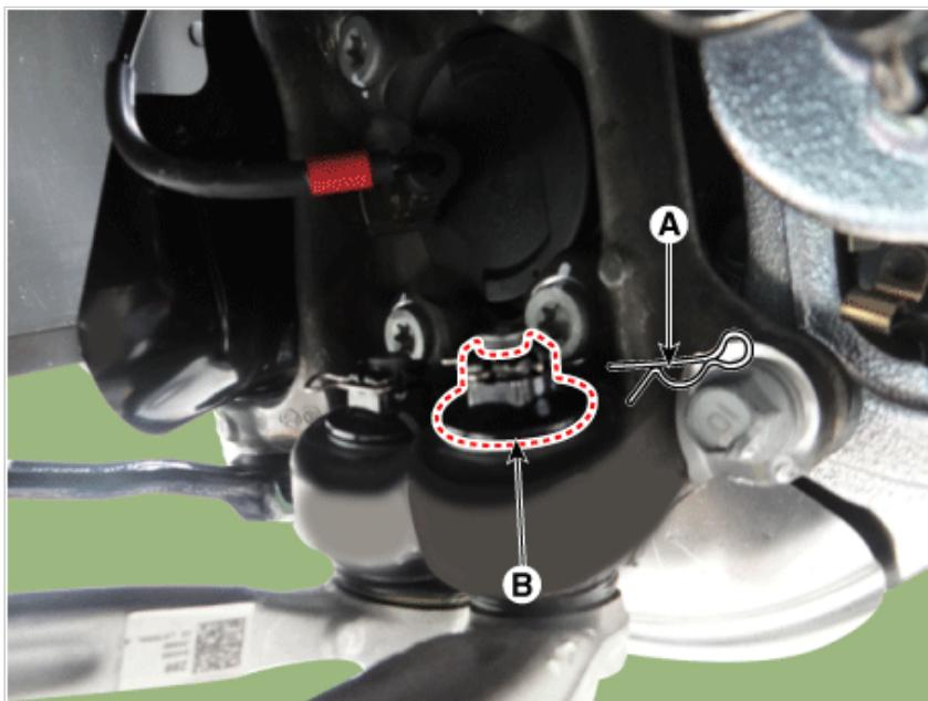
7. Loosen the compression arm bolt & nut from the sub frame.
