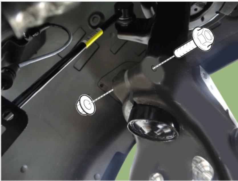
18. Remove the knuckle by using the SST (0K517-J5100).
