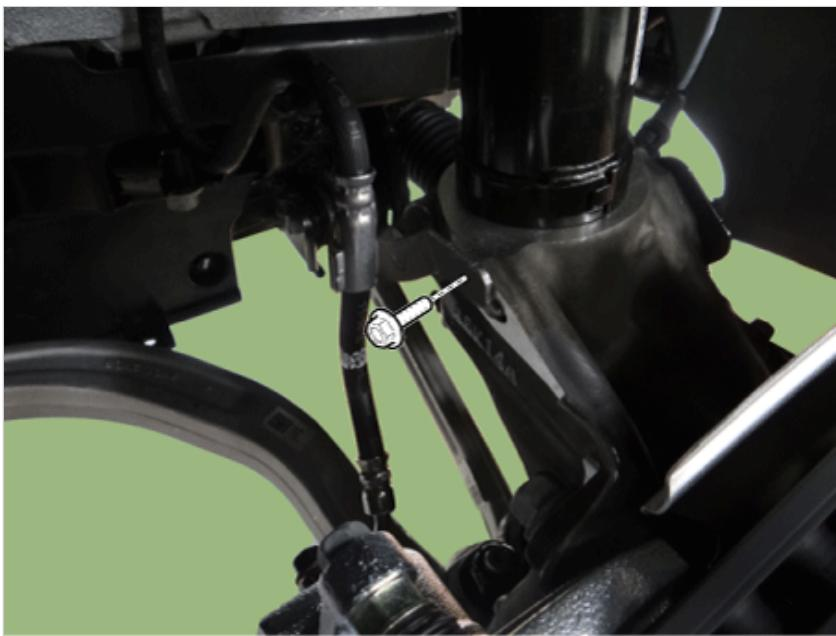
19. Loosen the brake cooling cover bolts.
