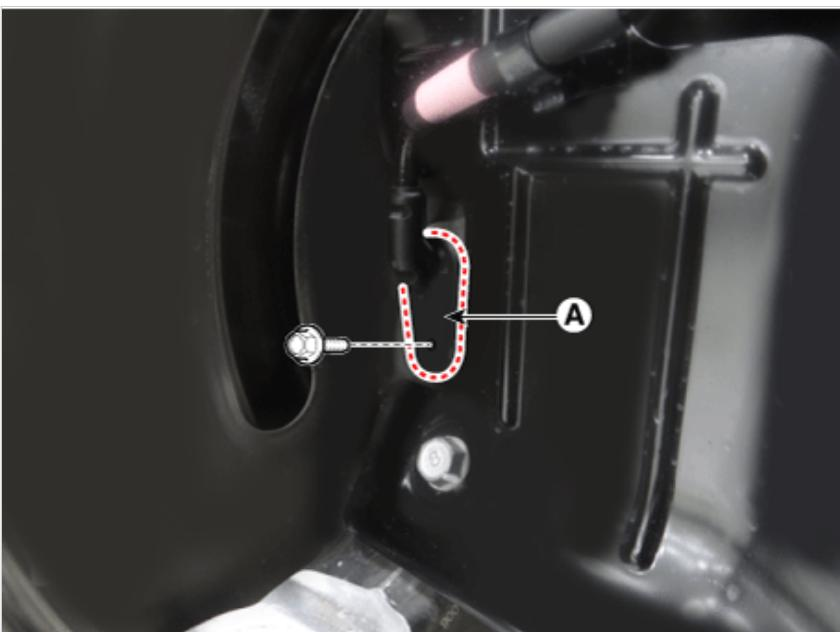
15. Remove the brake cooling cover (A).
