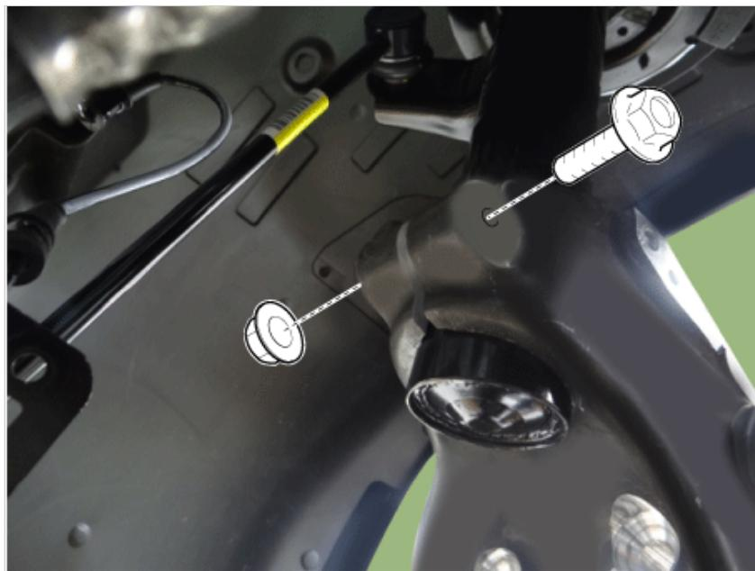
21. Remove the knuckle by using the SST (0K517-J5100).
