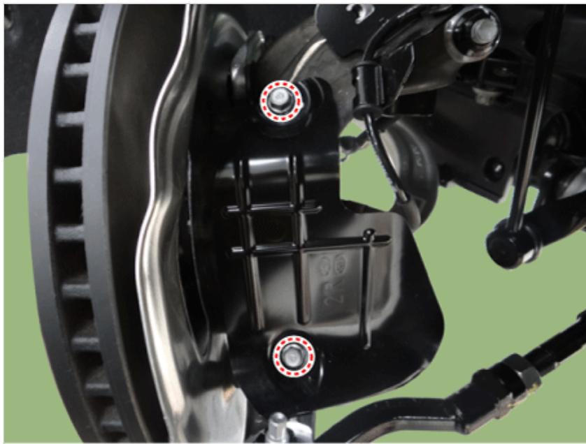
20. Loosen the knuckle upper bolt & nut.
