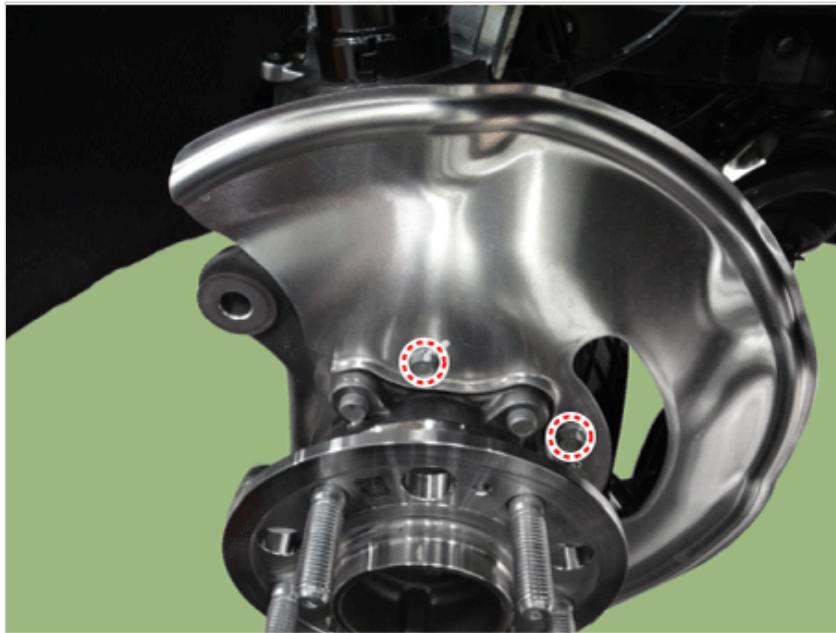
16. Loosen the hub assembly bolts and then remove the hub assembly.
